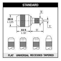
Available in 4 different end forms to place all fasteners (except Rivscrew). Suitable on applications with no or little access restriction.
