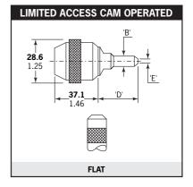
Available as shown in NOSE JAW SELECTION TABLE overleaf. Equivalent functions to the Standard and Limited Access above with the addition of a cam to ease and speed up the nose jaw opening thus the pod reloading procedure.
